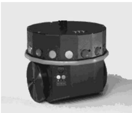
Fig. 17 Picture of the Nomad Scout robot with a differential drive mobile base.
