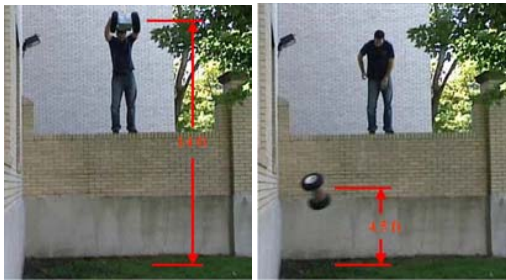
Figure 19: a) Initial Drop 4.3m (left) b) Rebound: 1.5m
