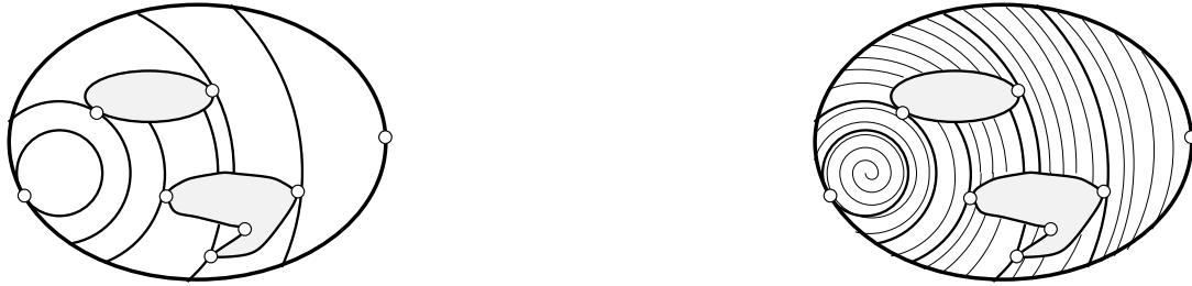
Fig. 12. Cellular decomposition for h(x) = (x_1)^2 + (x_2)^2 and an associated spiral coverage pattern. The slices are the circles that are the pre-images of h . At the critical points, demarked with little circles (not to be confused with the slices), the circle-shaped slices become tangent to the obstacles. Rather than moving along circular paths and stepping outward, the robot follows a spiral pattern.
