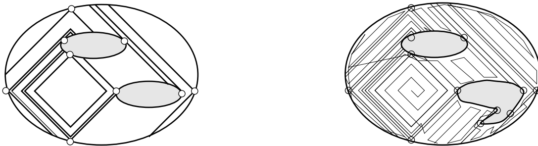
Fig. 14. Decomposition for h(x) = |x|_1 and a coverage pattern. Squares are the slices and at the critical points the corner of a square touches an obstacle and/or side of it becomes tangent to an obstacle. Since it is easier for the robot to move along straight lines rather than circles, this pattern can be used to approximate the spiral pattern.
