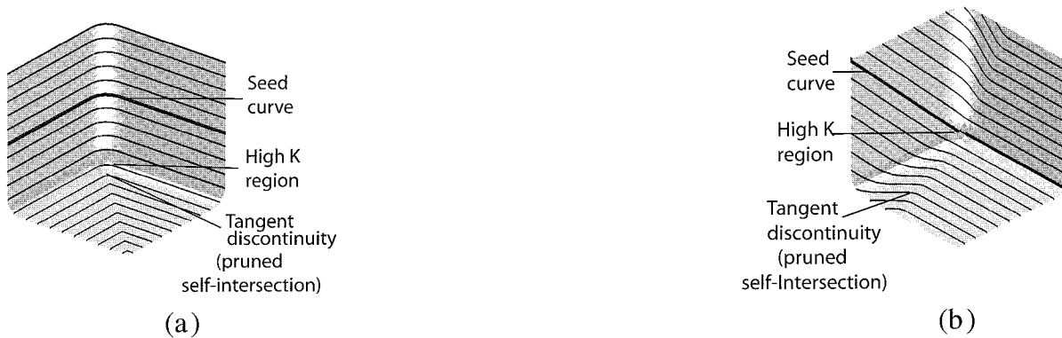
Fig. 7. (a) The geodesic curvature of offset passes increases as the passes sweep past a region of high Gaussian curvature. (b) If the seed curve (shown as a dark thick curve) splits the surface into two regions with equal integrals of Gaussian curvature, the geodesic curvature of the passes is minimized.
