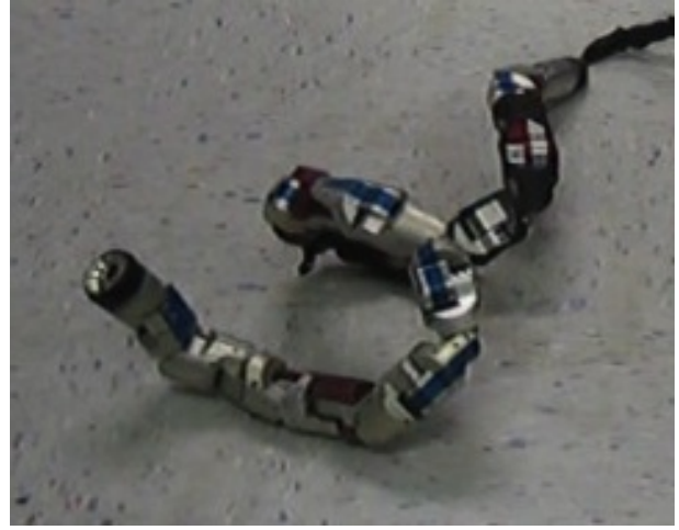
Fig. 8: This is the snapshot of our snake robot moving on a predefined path using conical sidewinding gait. It is currently forming a cone shape, and turning around our desired center.
