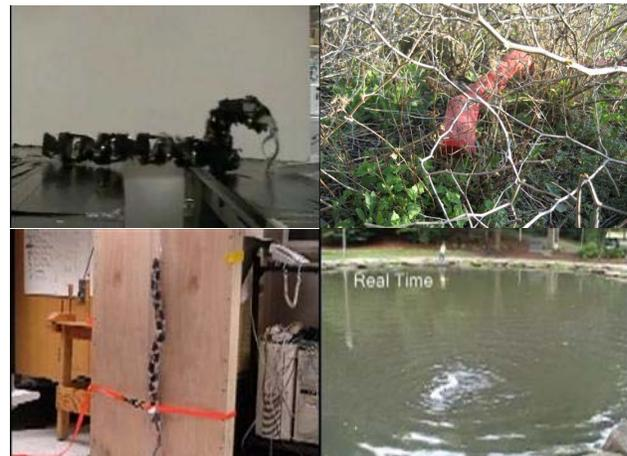
Figure 1: Our locomoting robots: reaching across a gap, traversing through brush, the inside of a pipe, and swimming.
