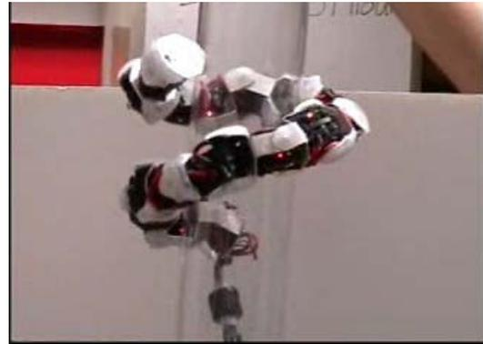
Figure 3: The snake robot forms a helix and climbs the outside of a pole.
