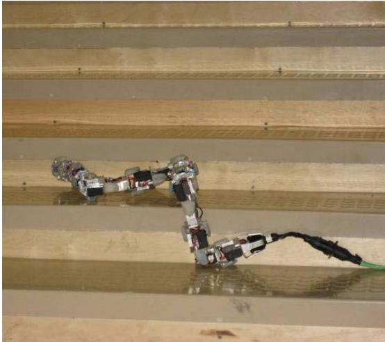
Figure 4: A snake robot using a piecewise differentiable stair climbing gait.
