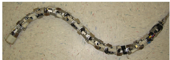
Fig. 10: Modsnake in its rolling “S” configuration
