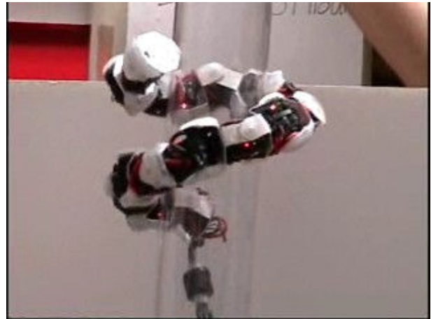
Fig. 1: Our modular snake ("modsnake") robots have sixteen joints, arranged to allow full workspace flexibility. In past work, we have demonstrated a variety of successful motion strategies for these robots, including traversal of both smooth and rough terrain, swimming, and pole climbing (shown here).
