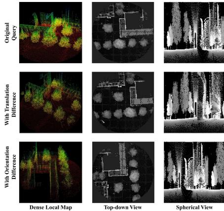
Fig. 2. **Different representations from local dense map.** Second and third row represent the same area under locally translation or orientation difference respectively. Different columns show the dense local map, the top-down and the spherical projections.
