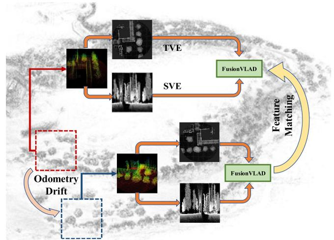
Fig. 1. **Fusion enhanced place recognition.** We generate multi-view projections from 3D point cloud, which are then fed into the proposed FusionVLAD network to extract global descriptors. Different projections (spherical view, top-down view) can capture different perspectives of the original 3D map.
