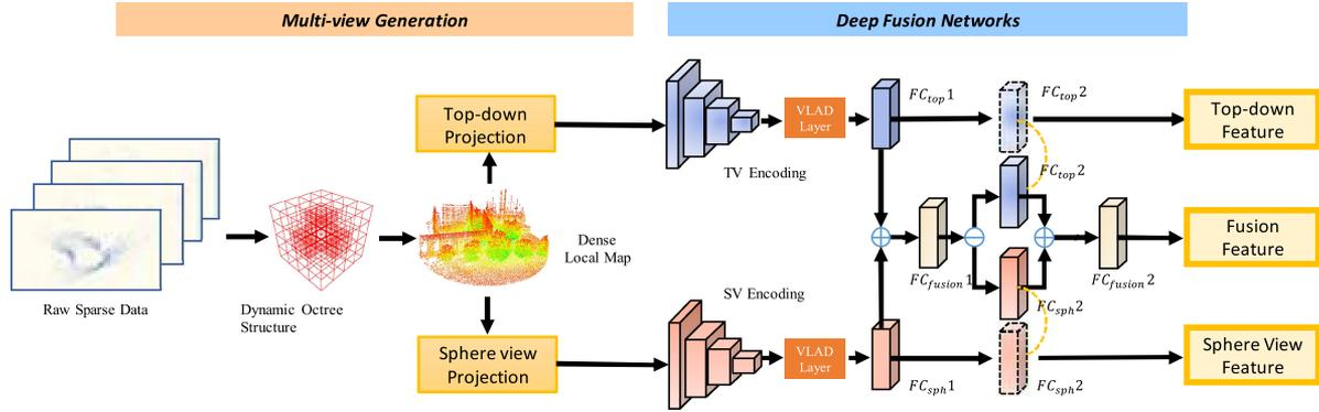
Fig. 3. **The network structure of our method.** Our FusionVLAD mainly includes two modules: Multi-view Generation module and Deep Fusion Networks module. With the given sequence of LiDAR scans, the first module can generate multi-view representations with the consideration of observation and odometry errors. The Deep Fusion Networks can parallel encode the top-down view and spherical-views, and tightly coupled the output features.
