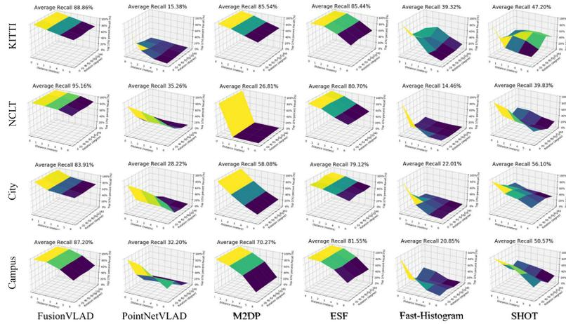
Fig. 6. Average Recall at Top 1% under variant viewpoint differences. Each sub-graph represent 16 trails of the place recognition average recall (z-axis) on different translation (x-axis) or orientations (y-axis). Each trail includes a reference trajectory and a testing trajectory (with translation/orientation noise).
