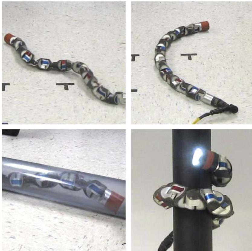
**Figure 1.** Examples of our snake robot executing the gaits discussed in this paper. From top left to bottom right: sidewinding, rolling, pipe crawling, and pole climbing.
