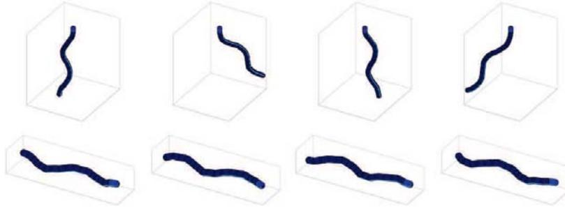
Fig. 4. A montage of the robot in sidewinding, shown in different positions from one gait cycle. The top row of images show the pose of the robot in a body frame fixed to the head link. The bottom row shows the pose corresponding to the virtual chassis body frame at the same points in the gait cycle.
