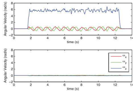
Fig. 6. A comparison of estimated angular velocities for the rolling gait, observed in a body frame fixed to the middle link (upper plot) and a body frame aligned with the virtual chassis (lower plot). The red, green and blue lines are respectively the  $x$ ,  $y$  and  $z$  body frame angular velocities.
