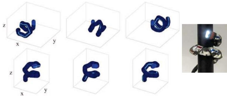
Fig. 2. A montage showing a snake robot at 3 positions in a gait used for climbing poles (right) viewed in a frame fixed to the head module (top row) and a frame aligned with the virtual chassis (bottom row).
