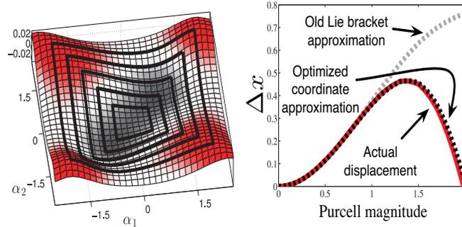
Fig. 5. Using the minimum perturbation coordinates greatly improves the accuracy of approximating the motion of a box stroke using the body velocity integral. Left, strokes of increasing magnitude in the shape space of the swimmer. Right, the displacement of the stroke shown in red, along with the approximation using a fixed frame (gray dashed) and minimum perturbation frame (black dashed).
