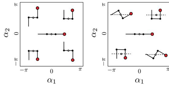
Fig. 1. Diagrams of the three-link swimming snake shown at zero orientation across corresponding shapes in a body frame fixed to the middle link (left) and a body frame defined by mean orientation (right).
