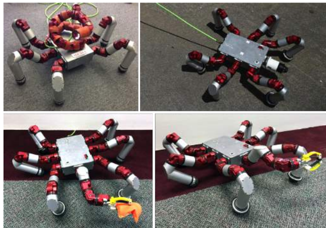
Fig. 1. Snake Monster (SM) with SEA Snake riding on its back (top-left). SM at the DRC Finals Expo using an IP camera head for live video streaming, object tracking, mapping, and navigation (top-right). SM configured with a 3-DoF arm and compliant, force-sensing, gripper (bottom).
