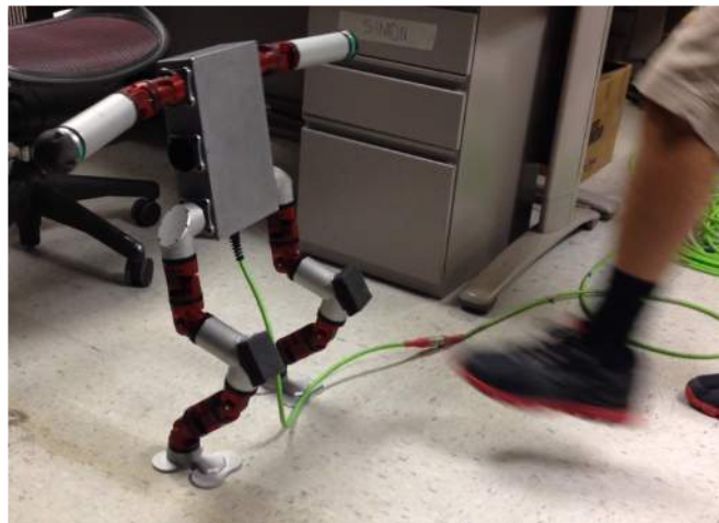
Fig. 8. Snake Monster Biped using ankle torque strategy and arm control to recover its balance from a kick.
