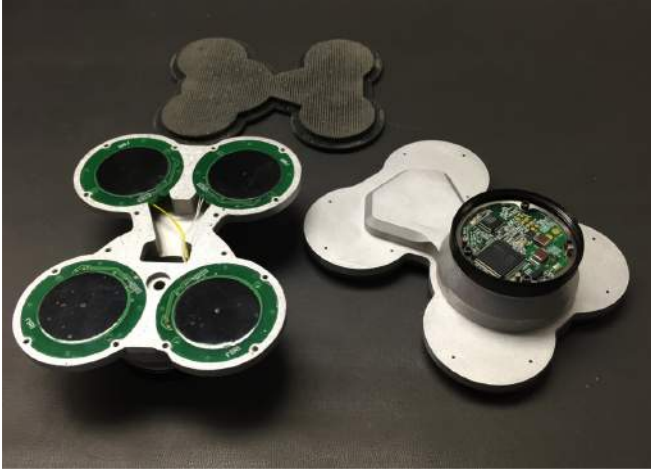
Fig. 6. Design of a lightweight (300 gram) multiple axis force sensing biped foot module.
