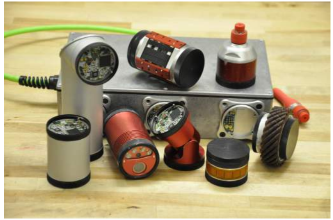
Fig. 3. Original SEA module and several other specialized actuation and sensing modules including tread, mecanum wheel, and 2-D Laser Distance Sensor Head modules among others.
