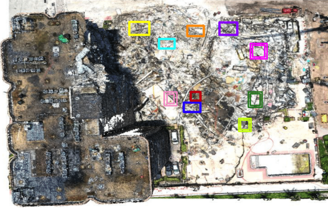
Fig. 3. Annotated regions corresponding to voids located in the collapse scene by experts. (Naturally occurring voids shown in double boundaries and voids created by excavation shown in single boundaries)
