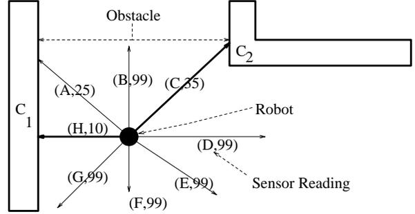
Fig. 4. Sensor Readings
