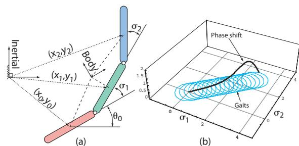
Fig. 1. (a) Coordinates describing the configuration of the three link snake robot. (b) Gaits proposed by Walsh[8].
