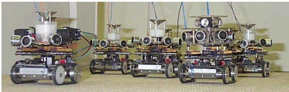
Figure 1: A team of Millibots exploring with sonar sensors
