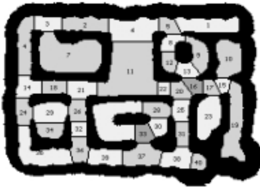
Fig. 14. Extracting the topological graph from the map depicted in Figure 9: (a) Voronoi diagram, (b) Critical points and lines, (c) regions, and (d) the final graph. (e) and (f) show a pruned version (see text).
