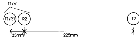
Figure 2 - Sensor arrangement, T=transmitter R=receiver V=vector receiver.
